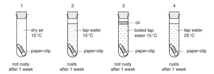
Which two experiments can be used to show that air is needed for iron to rust?
