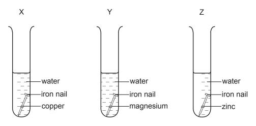
In which test-tubes will the iron rust?
