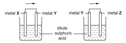
Which set of metals would give the electron flows in the directions shown?
