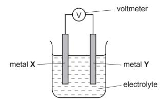
Which two metals produce the highest reading on the voltmeter?
