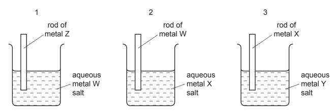
In beaker 1 metal W is displaced from solution.
