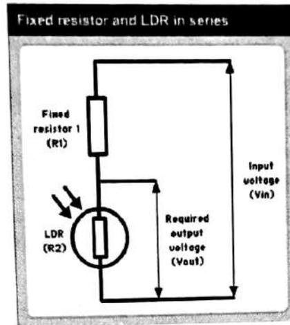
Figure 10: LDR used in a potential divider
