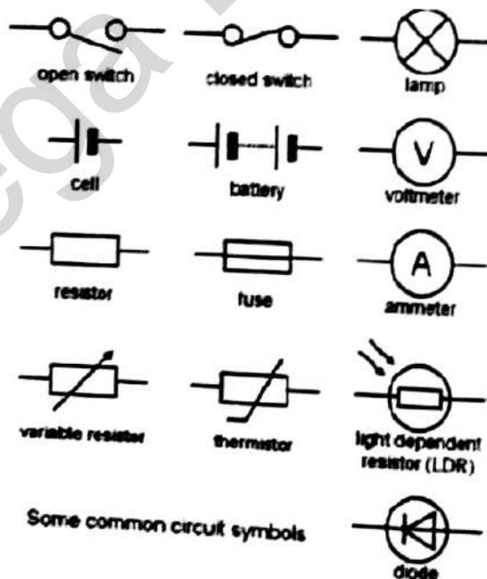
Figure: Symbols of common circuit elements
