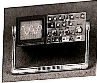
Oscilloscopes contain a vacuum tube with a cathode (negative electrode) at one end to emit electrons and an anode (positive electrode) to accelerate them so they move rapidly down the tube to the screen. This arrangement is called an electron gun. The tube also contains electrodes to deflect the electron beam up/down and left/right.
