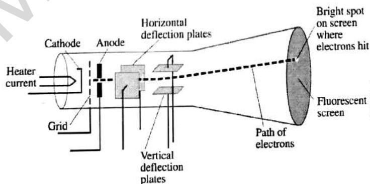
An oscilloscope is a test instrument which allows you to look at the 'shape' of electrical signals by displaying a graph of voltage against time on its screen. It is like a voltmeter with the valuable extra function of showing how the voltage varies with time. The 1cm grid enables you to take measurements of voltage and time from the screen.
