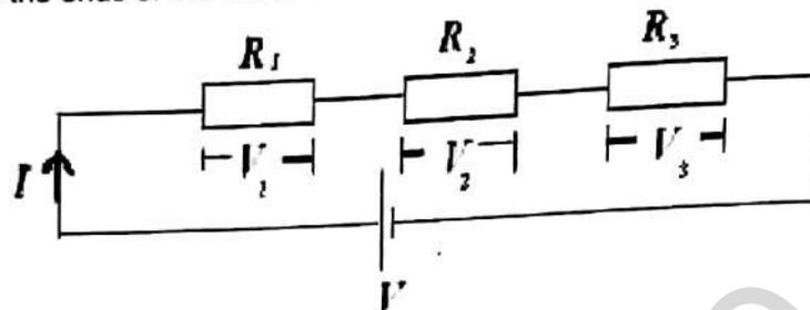
Figure Resistors in series-Note the current through all the resistors is the same but voltage is not. When a potential difference  $V$  is applied across the series the current through all the resistors is the same, but the potential difference across each resistor is different and the sum of these individual
