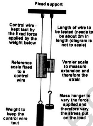
To minimize errors the control wire is the same length, diameter and material as the test wire. This means that errors due to expansion (from the surroundings) during the experiment are avoided as the test wire and control wire would both expand by the same amount and the scale would adjust position and eliminate the error.
