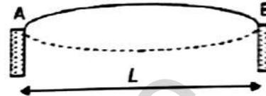
Hence, if the length of the bridge,  $L$ , is equal to  $\frac{1}{2}\lambda$ , the bridge will resonate with the fundamental frequency.
