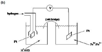
H<sub>2</sub> and good delivery system [1] Fe<sup>2+</sup>/Fe<sup>3+</sup> solution labelled [1] platinum electrodes (both) [1] salt bridge and voltmeter [1] H<sup>+</sup> or HCl or H<sub>2</sub>SO<sub>4</sub> [1] (acid is not sufficient)
