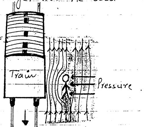
So between train and person streamlines are closer due to high speed, there will be low pressure exerted by fluid on person.
