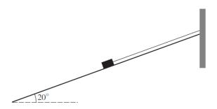
A block of mass  $8 \, \text{kg}$  is at rest on a plane inclined at  $20^{\circ}$  to the horizontal. The block is connected to a vertical wall at the top of the plane by a string. The string is taut and parallel to a line of greatest slope of the plane (see diagram).
