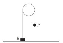
A block *B* of mass 5 kg is attached to one end of a light inextensible string. A particle *P* of mass 4 kg is attached to other end of the string. The string passes over a smooth pulley. The system is in equilibrium with the string taut and its straight parts vertical. *B* is at rest on the ground (see diagram). State the tension in the string and find the force exerted on *B* by the ground.
