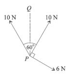
Three coplanar forces of magnitudes  $10 \,\mathrm{N}$ ,  $10 \,\mathrm{N}$  and  $6 \,\mathrm{N}$  act at a point P in the directions shown in the diagram. PQ is the bisector of the angle between the two forces of magnitude  $10 \,\mathrm{N}$ .
