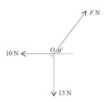
Three horizontal forces of magnitudes F N, 13 N and 10 N act at a fixed point O and are in equilibrium. The directions of the forces are as shown in the diagram. Find, in either order, the value of  $\theta$  and the value of F.
