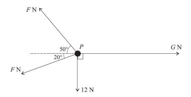
A particle P is in equilibrium on a smooth horizontal table under the action of horizontal forces of magnitudes F N, F N, G N and 12 N acting in the directions shown. Find the values of F and G. [6]
