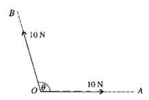
Two forces, each of magnitude 10 N, act at a point O in the directions of OA and OB, as shown in the diagram. The angle between the forces is  $\theta$ . The resultant of these two forces has magnitude 12 N.
