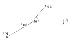
Three coplanar forces act at a point. The magnitudes of the forces are 5 N, 6 N and 7 N, and the directions in which the forces act are shown in the diagram. Find the magnitude and direction of the resultant of the three forces.
